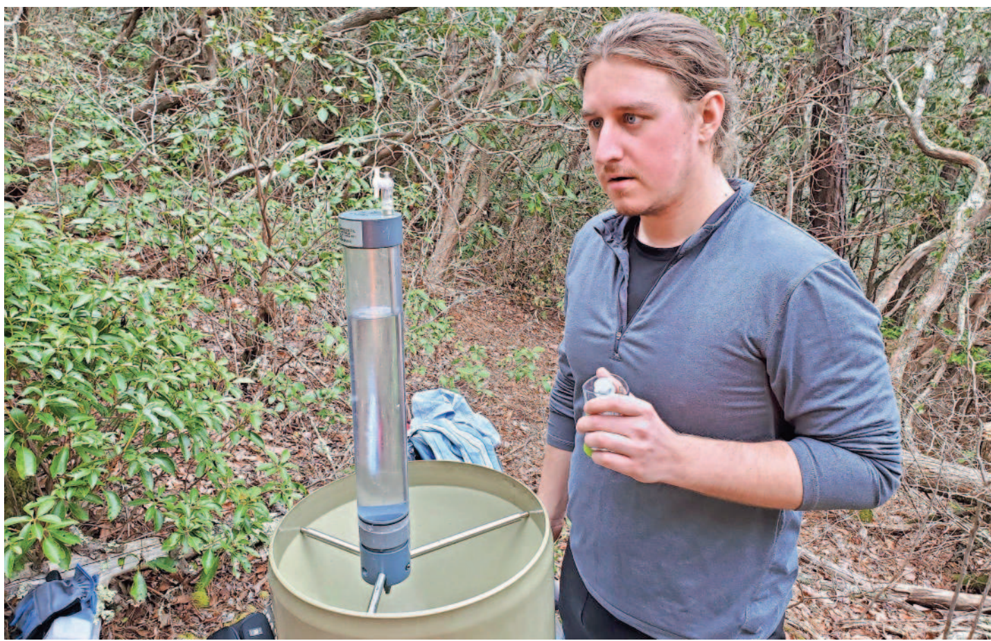
Mountain Rainger Samuel Peterson calibrates the rain gauge with a column of water. PHOTO PROVIDED
